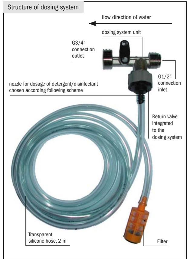
The dosage of detergent/disinfectant is done by nozzles in different sizes - supplied with the machine (Fig. 15). To achieve the desired concentration choose the corresponding nozzle (see below scheme).
