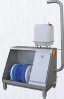
**Automatic sole washer with side cleaning, sanitiser dosing and drainage**
